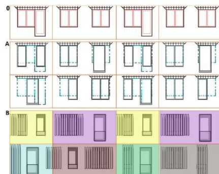
Fig. 12. Schematic of the location of the modules on the left side of the elevation [17] 0 - additional reinforcement of lintels with Helifix [12]; A – changes to the shape of openings; B – proposed pattern of façade modules on the example of two storeys with vertical covers made of lamellas
